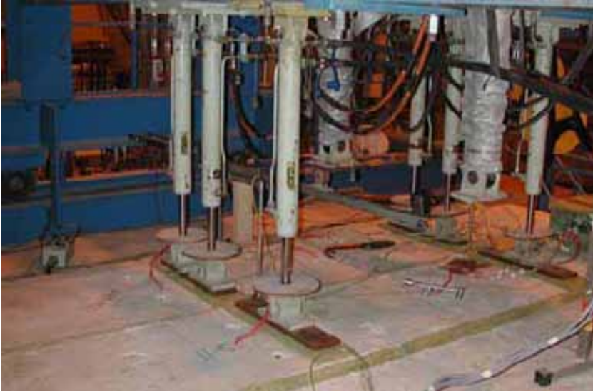
Figure 4.19 Beam specimens placed on the horizontal furnace.
