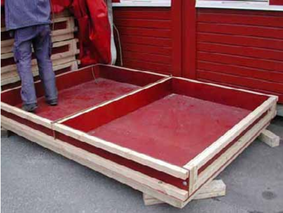
Figure 3.7 Mould for large slab specimens.
