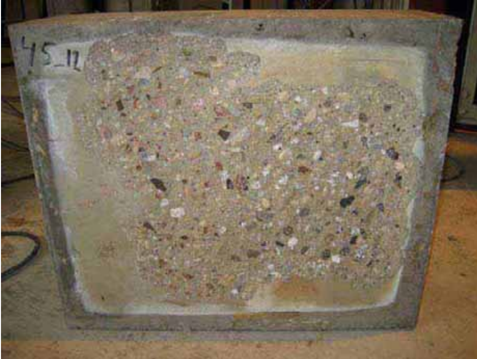
Figure A.523 Specimen 45-12 after test.
