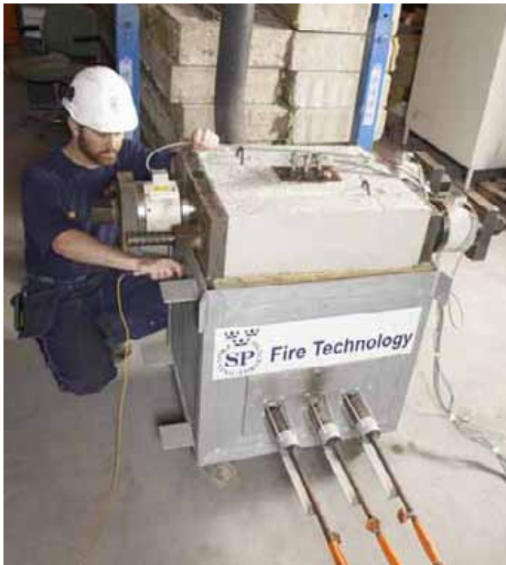
Figure 4.2 Small slab placed on the furnace.
