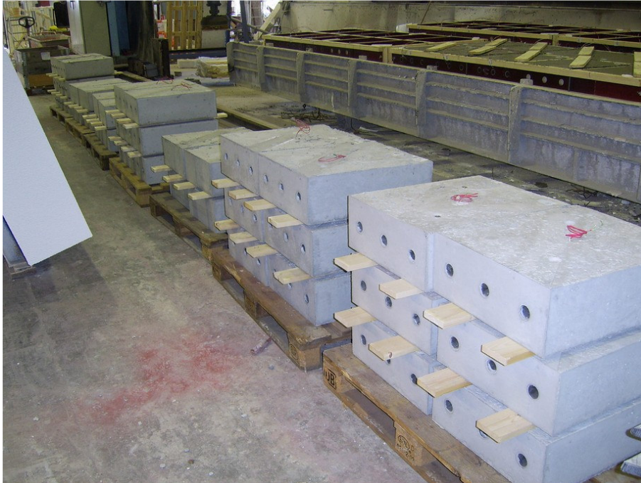
Figur 4-1 Mindre betongelement 500×600×200mm
