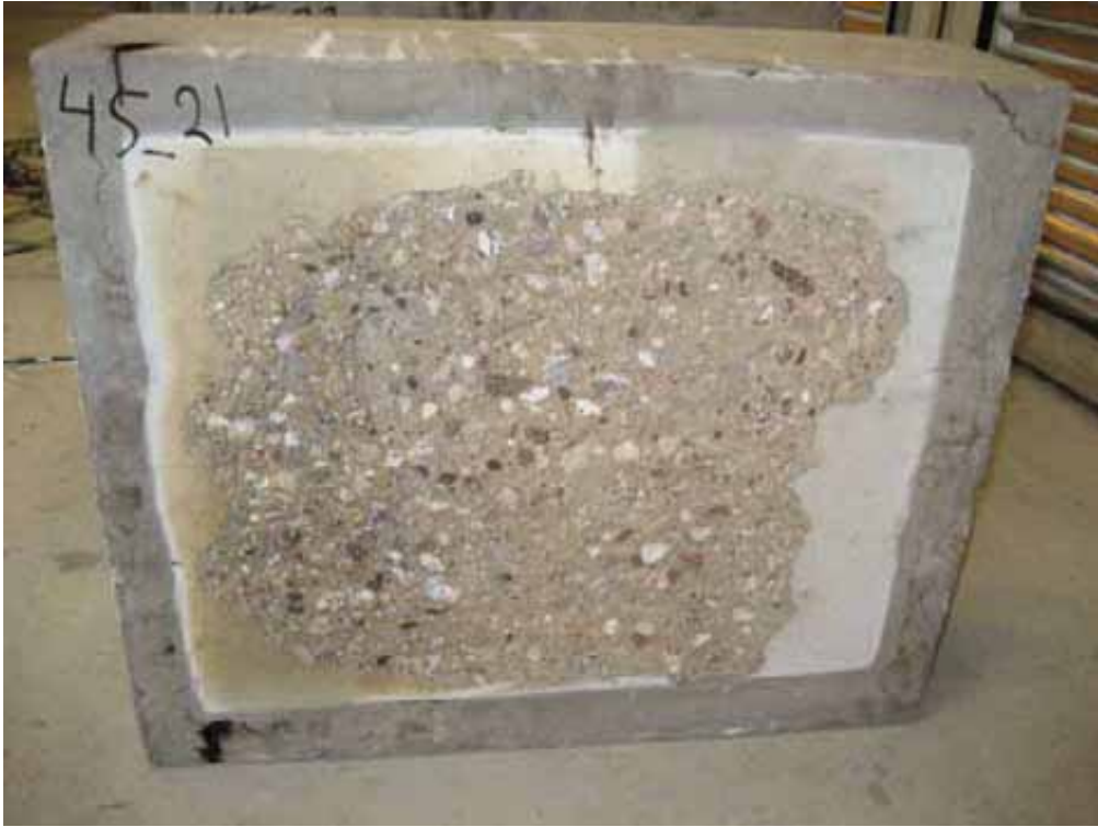
Figure A.543 Specimen 45-21 after test.
