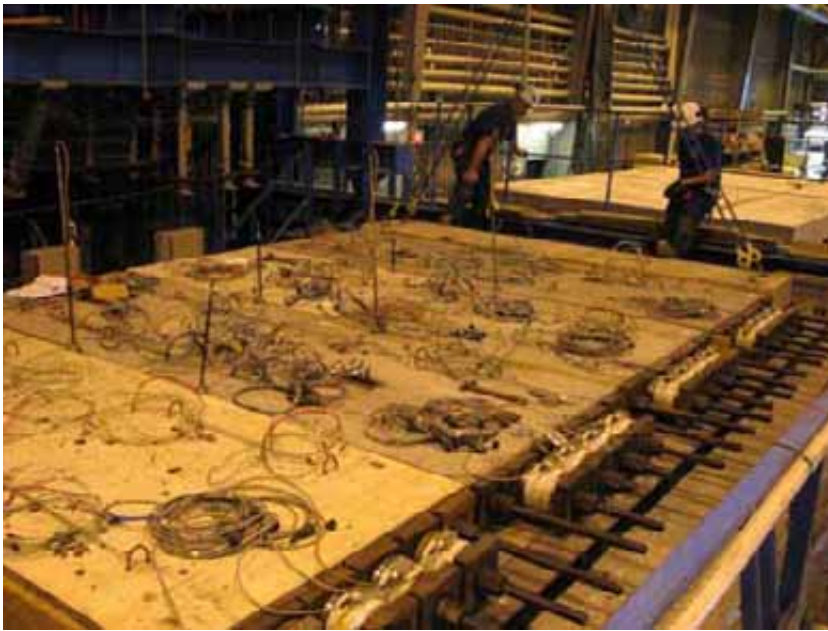
Figure 4.7 Slab specimens on the horizontal furnace.
