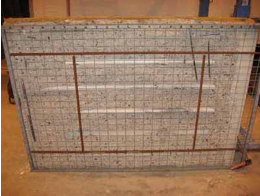
Figure 4.18 Specimen with a grid for spalling measurement mounted.
