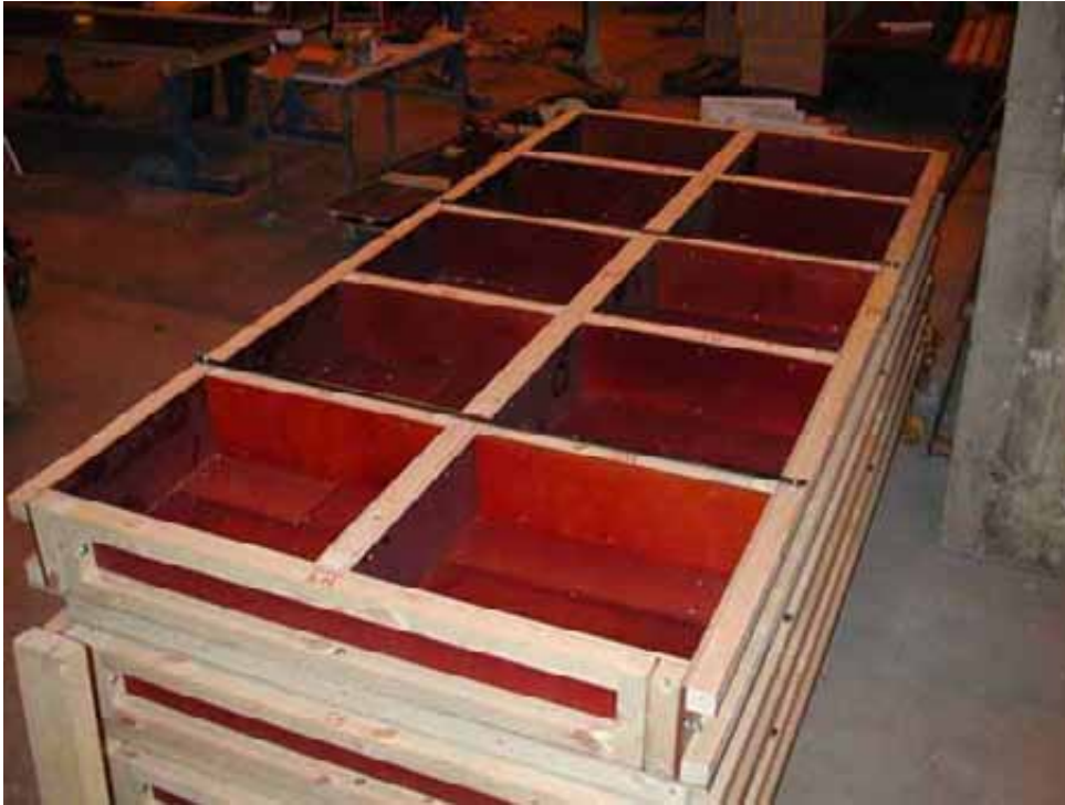
Figure 3.2 Moulds for small slab specimens.
