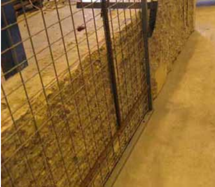
Figure 4.21 Grid for spalling measurement mounted on a beam specimen.
