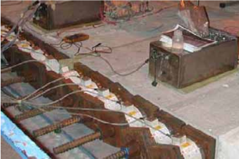
Figure 4.15 Load cells mounted between steel plates.
