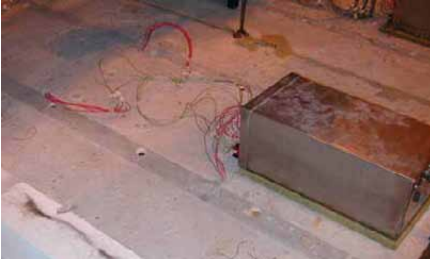
Figure 4.13 Temperature measurements in a concrete slab.
